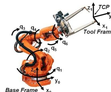
$$Z = \begin{bmatrix} \text{pos} \\ \text{ori} \end{bmatrix} = \Gamma_{kin}(q)$$
