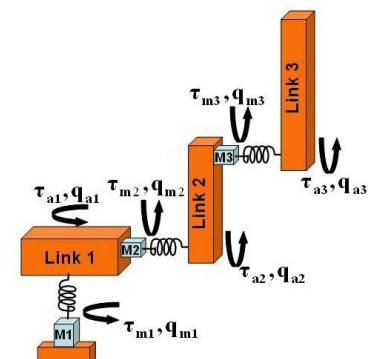
$$\begin{aligned} M_m \ddot{q}_m + \tau_{fm}(\dot{q}_m) + r_g \tau_g &= \tau, \\ M_a(q_a) \ddot{q}_a + c_a(q_a, \dot{q}_a) + g_a(q_a) &= \tau_g, \\ k_g(r_g q_m - q_a) + d_g(r_g \dot{q}_m - \dot{q}_a) &= \tau_g, \end{aligned}$$
