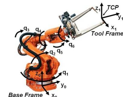
$$Z = \begin{bmatrix} \text{pos} \\ \text{ori} \end{bmatrix} = \Gamma_{kin}(q)$$
