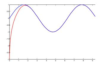
Figure 11.4: Series connection of circuit model and its inverse. Reference signal starts at 0 and output at -3.
