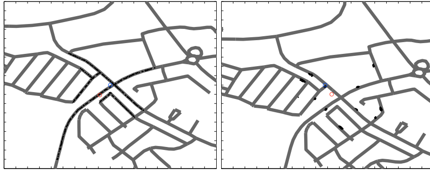
(a) The PF is depicted shortly after initialized (b) Multi-modal PDF representing the positioning prior information.
