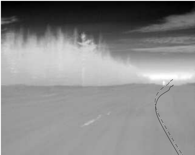
Fig. 2. The vehicle motion estimates (solid: from smoothing, dash-dotted: from filtering) are here reprojected into an image.
