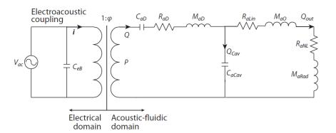
It is therefore proposed to use lumped element modeling (LEM) that is combined with equivalent circuit representations to estimate the nonlinear dynamic response of a synthetic jet as a function of device dimensions, material properties, and external flow conditions. Former work has been performed by for example Ref [1] giving promising results using this methodology.
