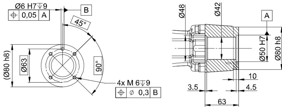
Figure 21 Robot tool flange for IRB 1600ID-4/1.5 (dimensions in mm).
