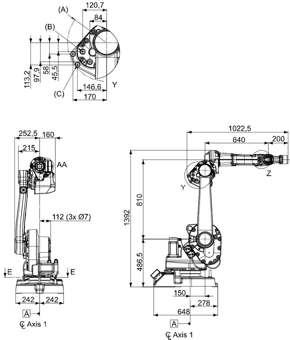
Figure 19 Holes for mounting extra equipment on the wrist, the upper arm housing and on the frame of IRB 1600ID-4/1.5.
