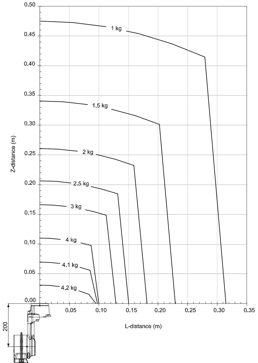
Figure 14 Maximum permitted load mounted on the robot tool flange at different positions (center of gravity)
