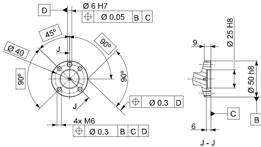
Figure 20 Robot tool flange (dimensions in mm).
