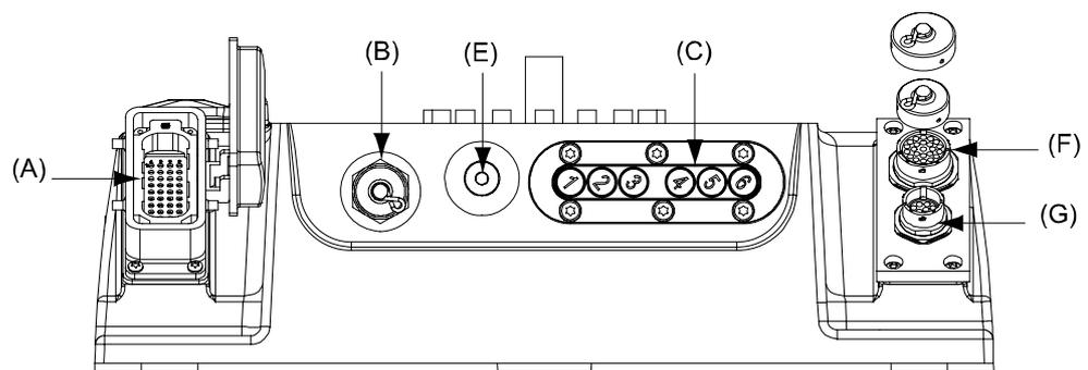
Figure 29 Integrated wirefeed interface.
