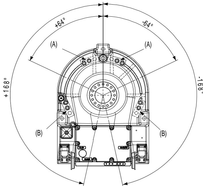
Figure 32 Mounting area of the additional stops for Axis 1.
