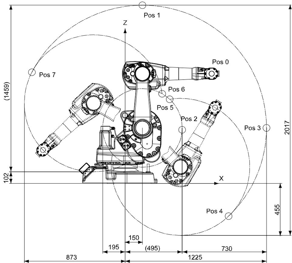
Figure 22 The extreme positions of the robot arm with 1.2 m reach.
