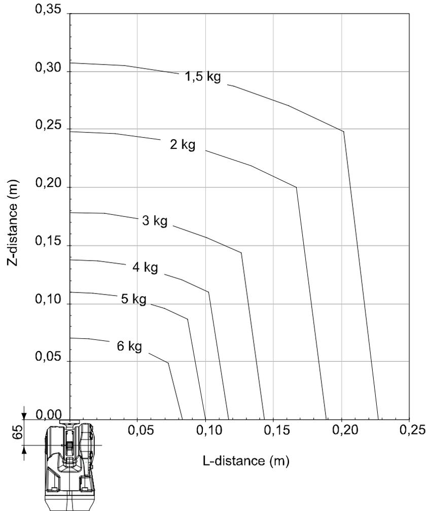
Figure 10 Maximum permitted load mounted on the robot tool flange at different positions (center of gravity).
