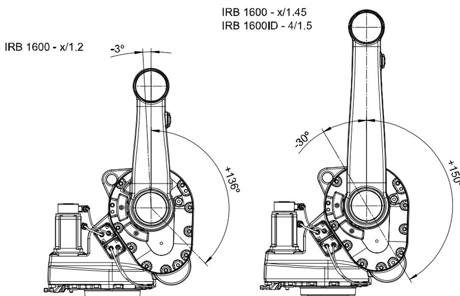
Figure 34 Mounting area of additional stop Axis 2.
