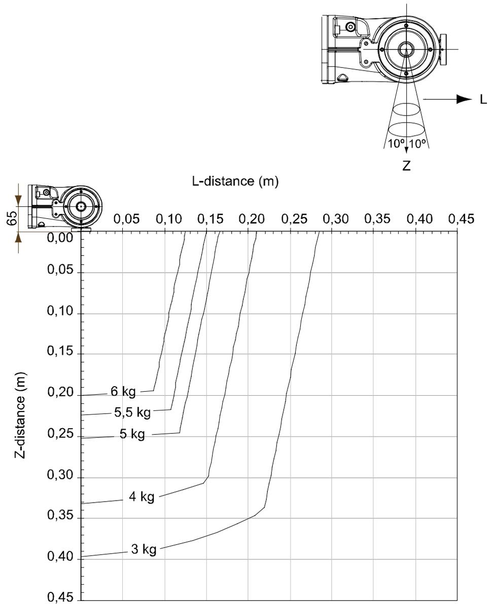
Figure 11 Maximum permitted load mounted on the robot tool flange at different positions (center of gravity) at “Vertical Wrist” ( $\pm 10^\circ$ ).
