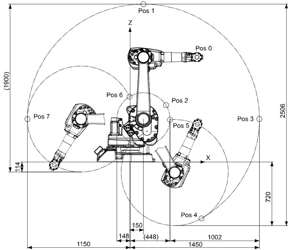
Figure 23 The extreme positions of the robot arm with 1.45 m reach.
