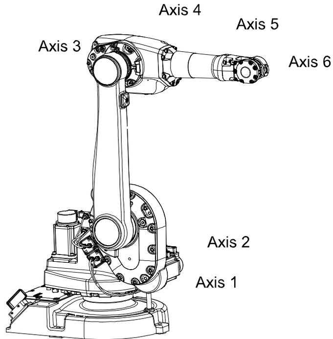
Figure 8 All axes in zero position.
