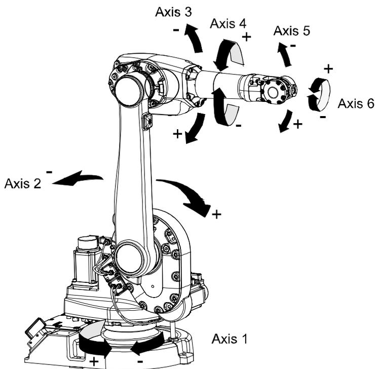
Figure 1 The IRB 1600 manipulator has 6 axes.
