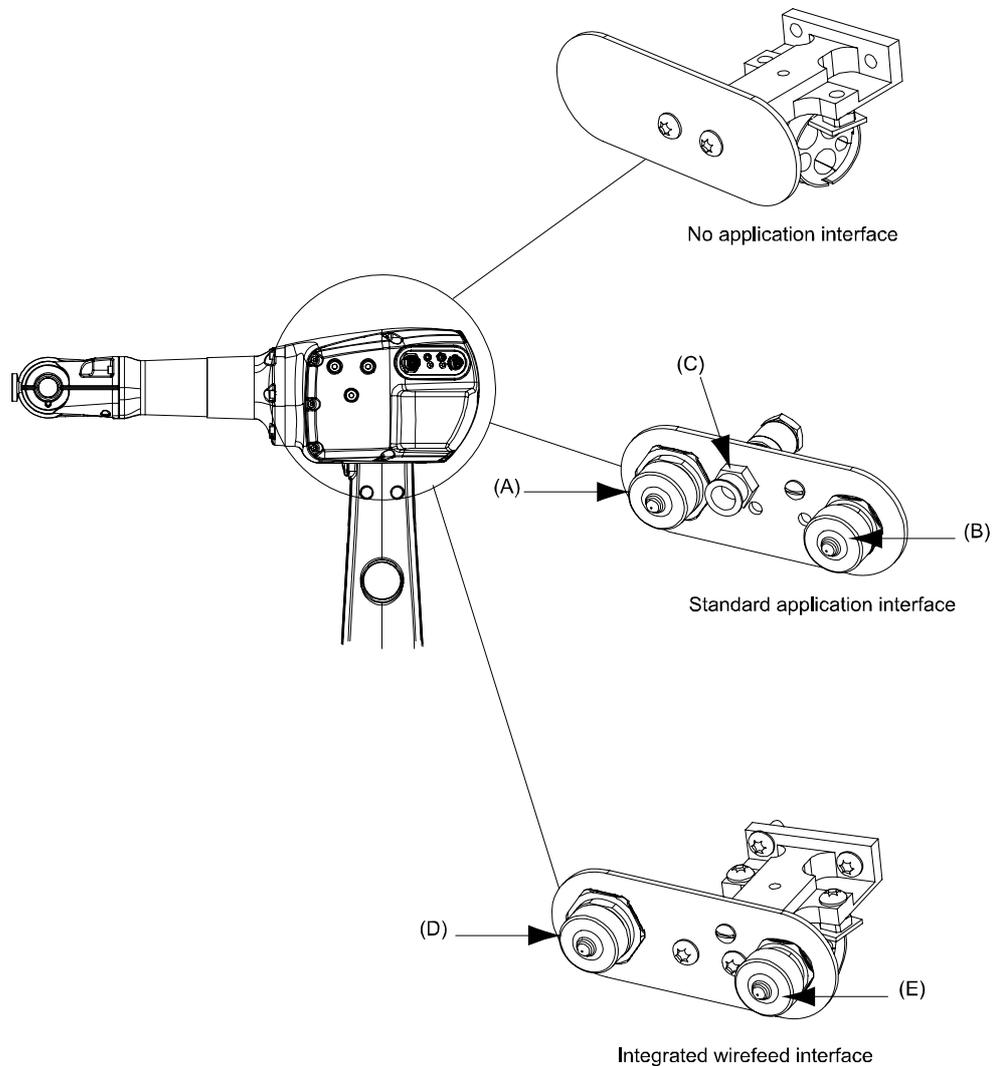
Figure 31 Customer connections at the upper arm.
