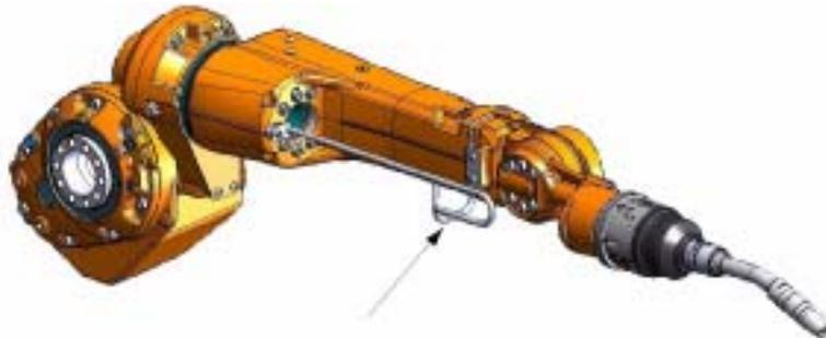
Figure 36 Process cable protection to be mounted on the upper arm.
