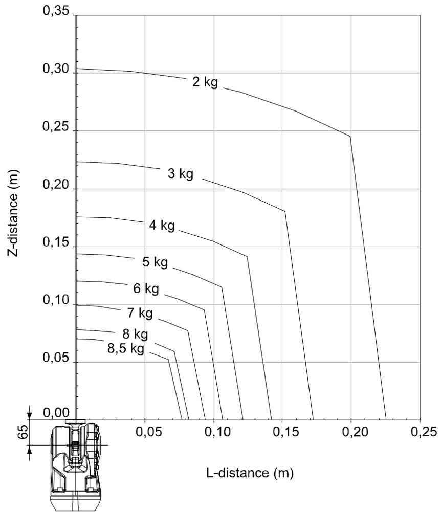
Figure 12 Maximum permitted load mounted on the robot tool flange at different positions (center of gravity).
