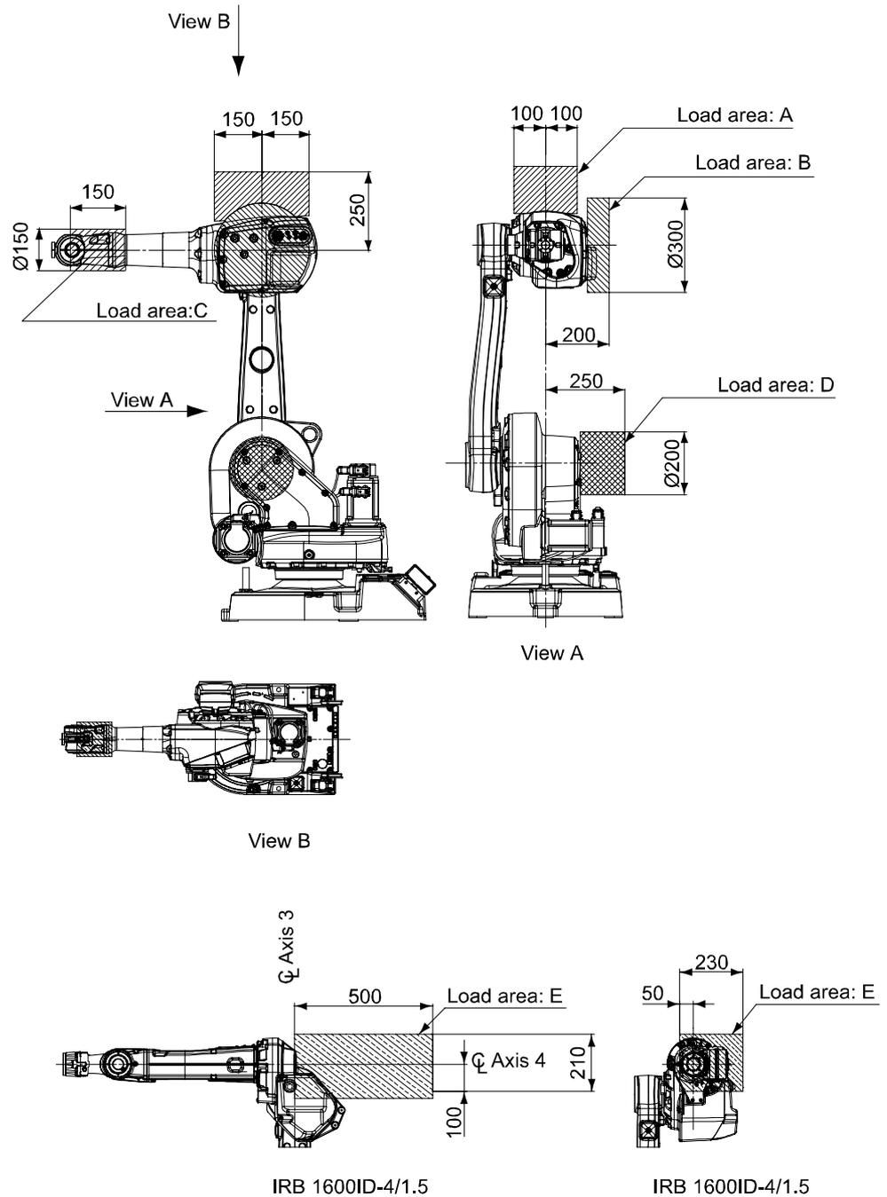
Figure 17 The shaded area indicates the permitted positions (center of gravity) for extra load mounted on the robot (dimensions in mm).
