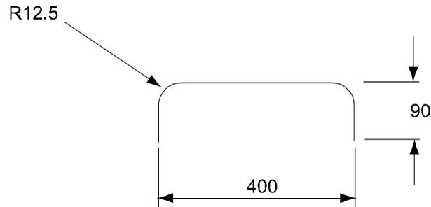
Figure 26 Packer cycle (dimensions in mm).
