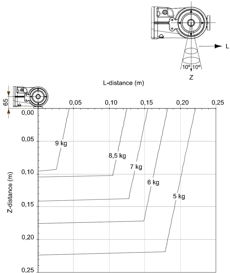
Figure 13 Maximum permitted load mounted on the robot tool flange at different positions (center of gravity) at “Vertical Wrist” ( $\pm 10^\circ$ ).
