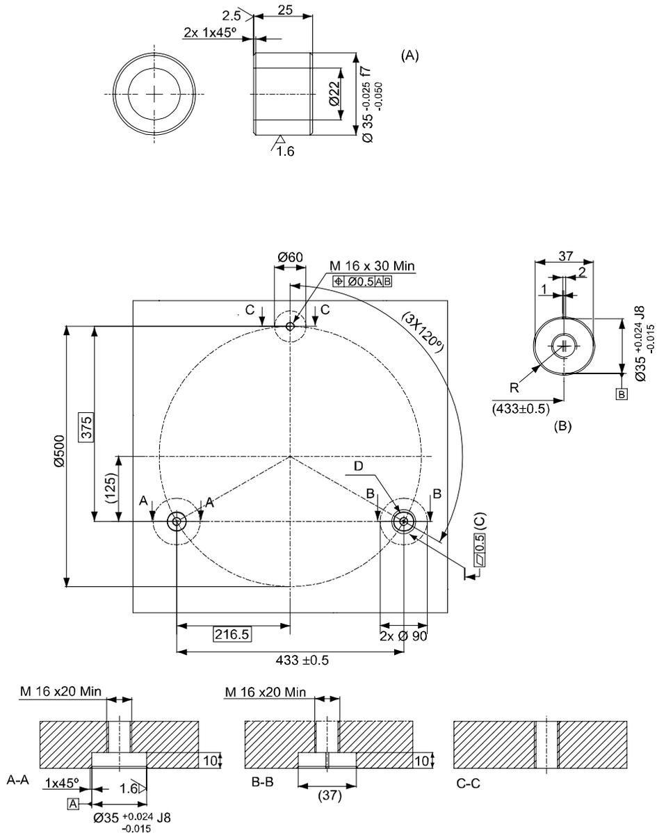
Figure 7 Mounting surface and bushings.
