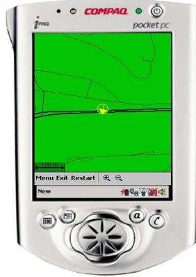
Figure 5.2: The car navigation system MAP (NIRA Dynamics AB) is based on particle filtering using wheel speeds and street map as only information.
