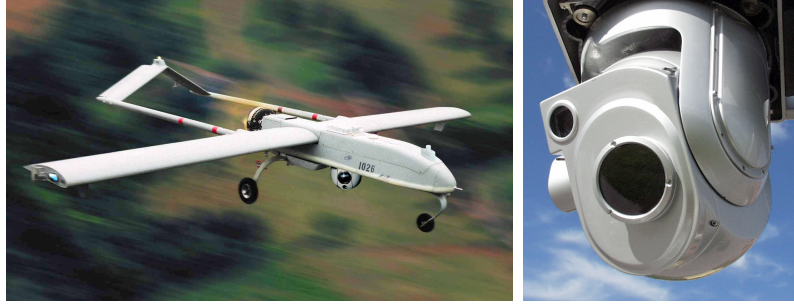
Figure 4.3: Left: example of an unmanned aerial vehicle, here a RQ-7 Shadow UAV. Right: example of a gyro-stabilized sensor gimbal with an infrared sensor. The gimbal has two actuated DOFs, pan and tilt.
